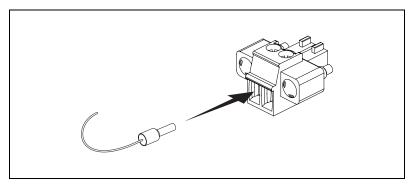
Figure 7. 2-Terminal Detachable Screw-Terminal Connector with Ferrule
